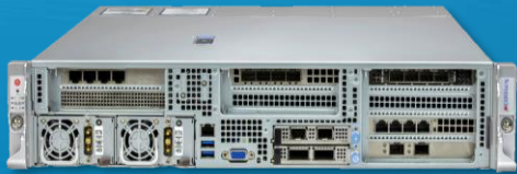
2U Hyper-E Short-Depth (Up to 3 DW GPUs or 4 SW GPUs) SYS-221HE-FTNR, SYS-221HE-FTNRD
