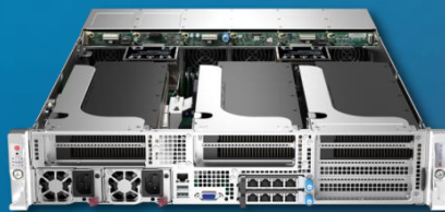
2U Hyper-E Short-Depth (Up to 3 DW GPUs or 4 SW GPUs) SYS-221HE-FTNR, SYS-221HE-FTNRD
